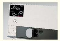
paper stop with sensor activates the punching cycle
