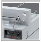
Transparent safety guards made from unbreakable plastic on front and rear table: The hinged front safety guard locks in the lower position while cutting.
